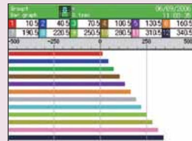
Bar-Graph Screen Display data (measured and virtual) of selected group. Combination display with real-time trend is available.
