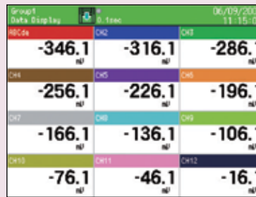
Data Screen Display data (measured and virtual) of selected group. Simultaneous display of alarm status.
