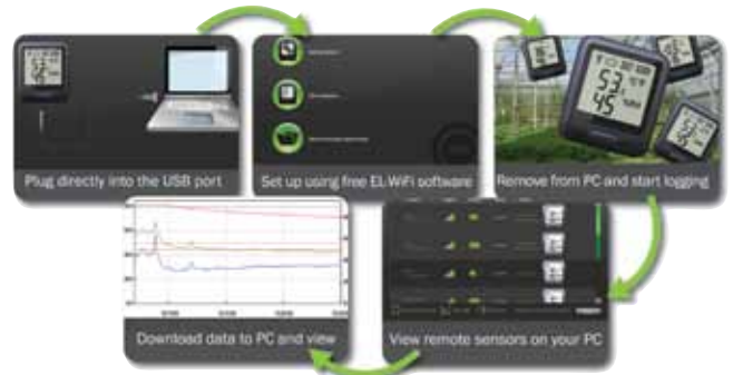
Windows® software used for data logger set up, data transfer and display. (Software available free at OMEGA)
