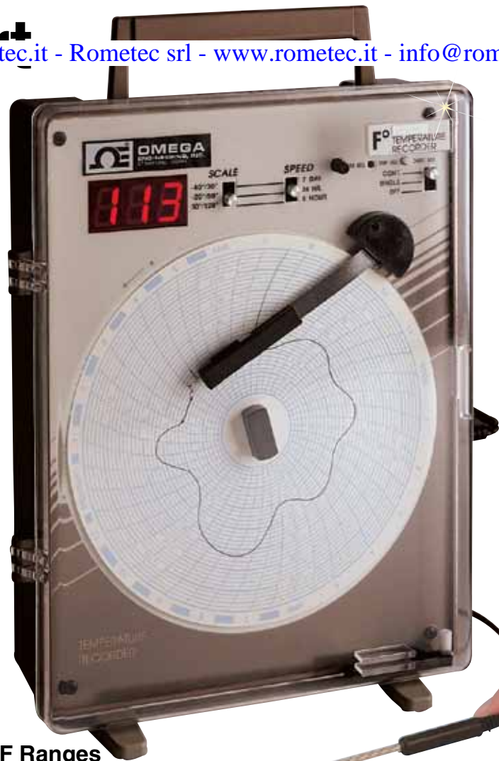
CT87LF low temperature recorder, with CT87-J-NP probe (included with the CT87L models).
