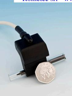
This high performance low-flow miniature turbine meter provides instantaneous response even at extremely low flows. Featuring photo-electric sensing, the AVi is constructed from chemically inert materials making it suitable for many liquid and trace chemicals. The rotor is near weightless in liquid meaning there is negligible bearing wear. Available in frequency output, the meter offers instantaneous, batch and totalised flow measurement.
