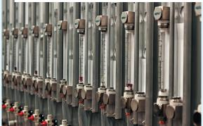
Each flowmeter scale is produced using our bespoke air or water calibration facilities where all reference equipment used is traceable to national standards and controlled within our approved ISO9001:2008 management system, assuring accuracy within the required limits.
